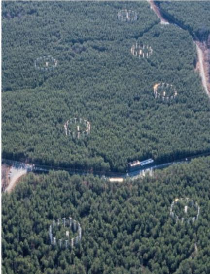
**Fig. 1.** Free-air CO<sub>2</sub> enrichment (FACE) rings in a pine plantation in North Carolina, USA. Each ring is 30 m in diameter and circumscribes about 100 trees. The distance from the single ring in the southwest (top right) to the two rings in the north (bottom) is ~500 m. The single ring in the background is a prototype. There are six experimental rings; three rings receive ambient air and three receive ambient plus 200 μl liter<sup>-1</sup> CO<sub>2</sub> (photo: Will Owens).
